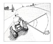
Only Hydro-Clipper has the 90° self-returning breakaway feature, which makes it unnecessary for the operator to leave the tractor seat to reposition the cutterbar after striking an object. It is trouble free and requires no maintenance. When mowing brush, vetch, etc., the tractor clutch is not slipped as is necessary with a spring-loaded latch-type breakaway.
