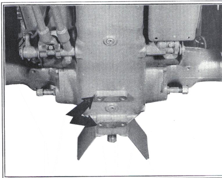
Effective with Super 55 tractor serial number 52 814-519 a new swinging drawbar has been released. This drawbar assembly is not interchangeable with previous Super 55 tractors due to the method of attachment to the rear frame.
