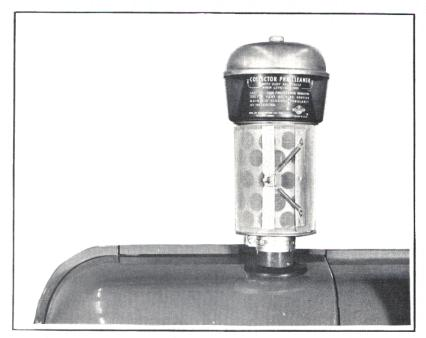
Effective approximately October 1, 1957, Air Intake Precleaner Screener Field Installation Packages will be available for Fleetline 77 Diesel, Fleetline 88 HC and Diesel, Super 77 and 88 HC and Diesel, and Super 55 Diesel tractors. These precleaner screener packages are made available to meet field demand where adverse dust and plant fiber lint conditions exist.
